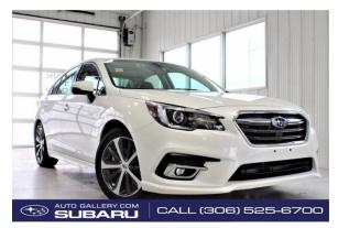
The Legacy 3.6R uses Active Grille Shutter on the front of the car to help improve fuel economy. Upon startup, it closes to warm the engine up faster, and while driving, it closes to reduce wind resistance and cold airflow. However, when the engine becomes hotter, it opens to cool off the engine. Unleash the power within to pursue what you want most. The 2019 Legacy connects you to the thrill of driving with an engaging, responsive ride and AWD capability to get you where you need to go with
